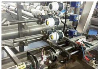
Magnetic flowmeter in calibration
