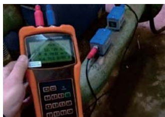
Ultrasonic flow meter for clean water measurement
